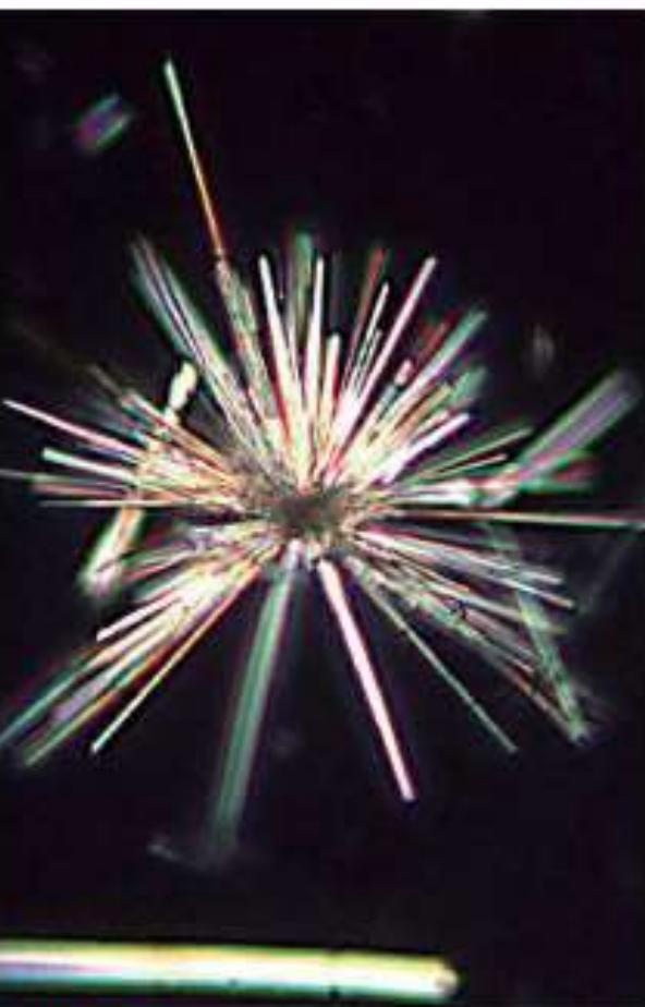
FIGURE 3.7 A "star-like" crystal and "needles" of ciprofloxacin (phase contrast, x 256).
