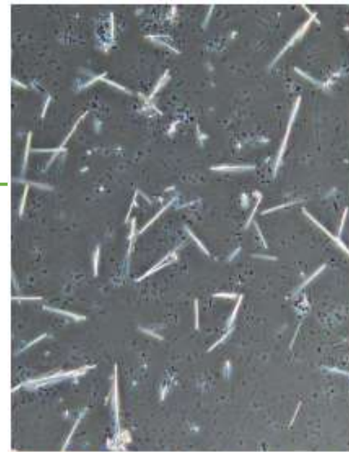
FIGURE 3.9 Many "needles" of ciprofloxacin (phase contrast, x 160).
